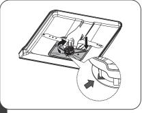
Reassemble the filters in the reverse order of the disassembly, replace the filter insert, and rotate clockwise to the close arrow.
