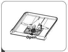
1 Hold the coarse filter and rotate it anticlockwise to unlock the filter. Lift the filter upwards and out of the dishwasher.
